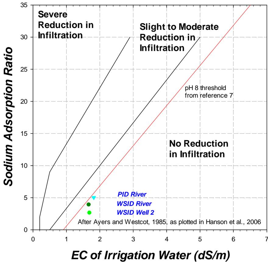
Figure 1. Salinity and SAR data plotted relative to infiltration sensitivity.
